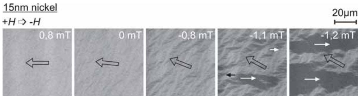
(b) The domains, switching from positive to negative field, recorded at 15 nm nickel thickness.
